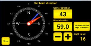
In the screen compass, red pointer shows the set blast direction, and the blue pointer shows current carrier direction derived from mounted GNSS Compass.
