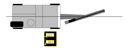
In **relative mode** both angles are related to the preset angles. This function makes it very easy to drill parallel holes:
