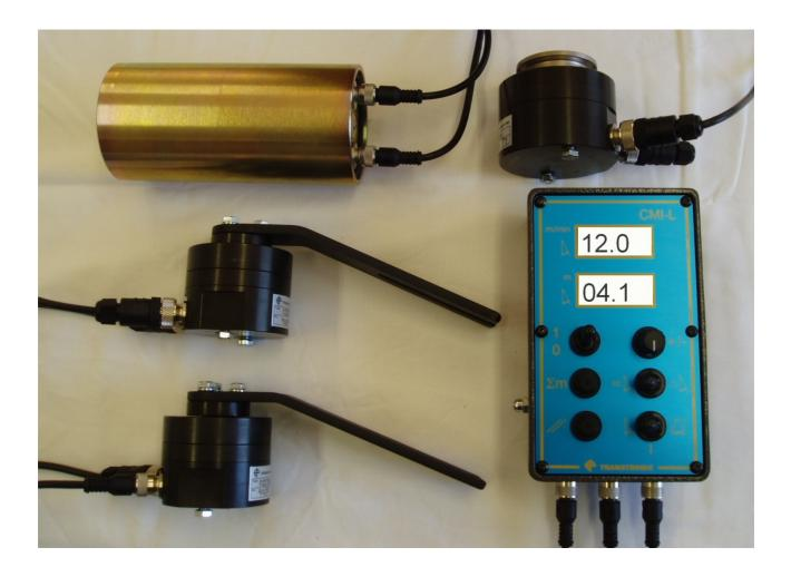
The picture shows one CMI Tunnel vertical and horizontal angle measurement and length measurement. (Cylinder feeder)
