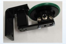
The length transducer measures length of movement through the rotation of its friction wheel, Laying against a rotating pulley wheel or a linear movement.
