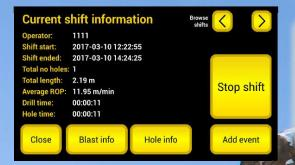
The user can manually add free text (events) during drilling to be saved with current shift and hole data. The saved data can be exported from the app database at any time to a semicolon separated file (csv) which can be opened and read with a spreadsheet application (see images below).
